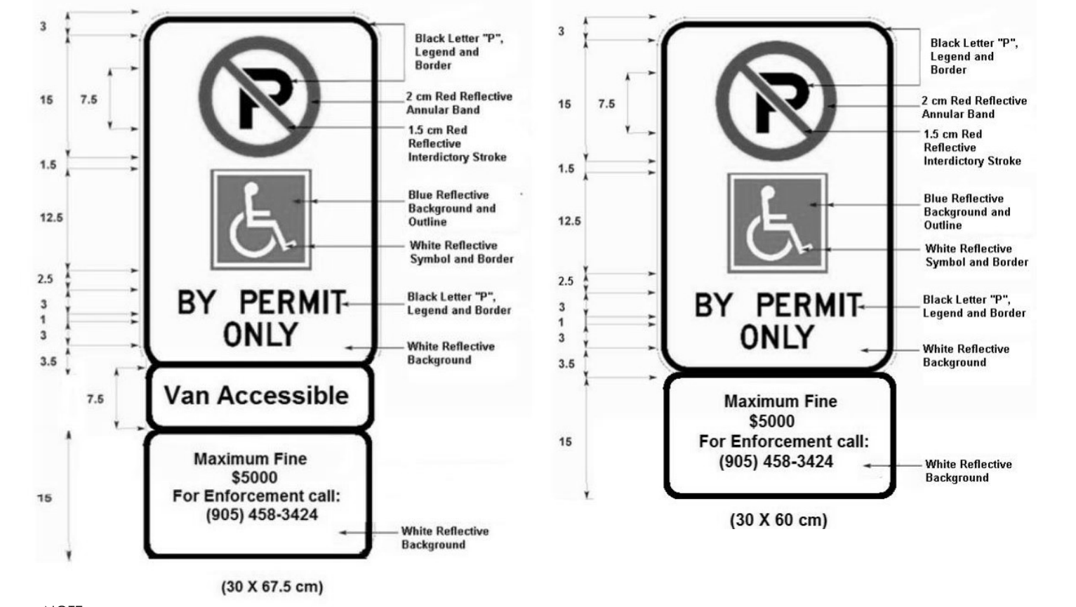
11.4 ACCESSIBLE PARKING SIGN DETAIL N.T.S.
