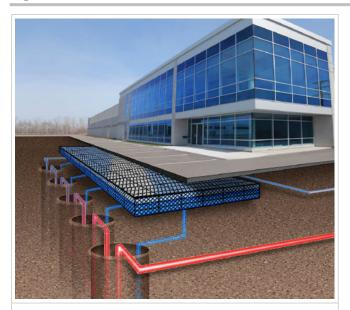
Figure D05.1- Ground Source Heat Loop
