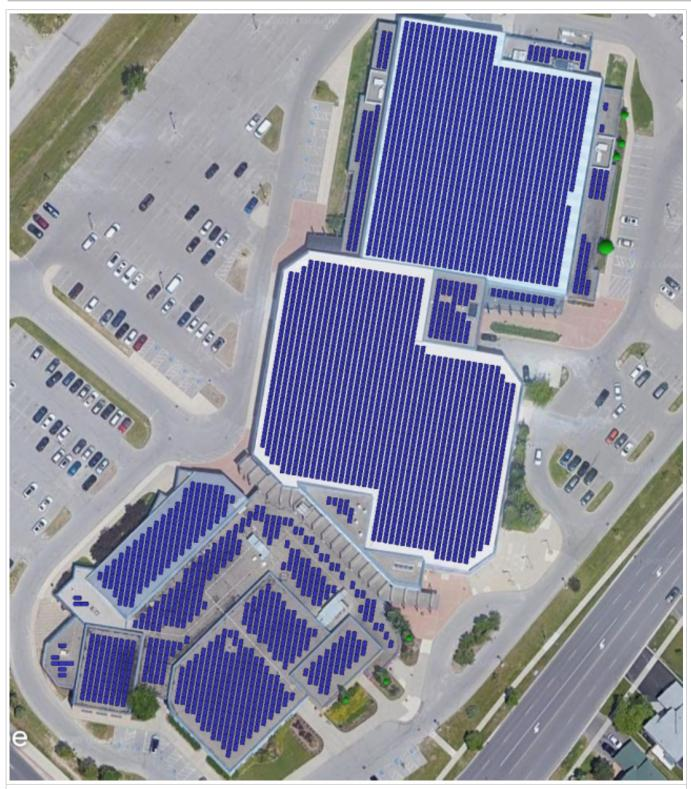
Figure IO1A. 1: Helioscope rendering of proposed array
