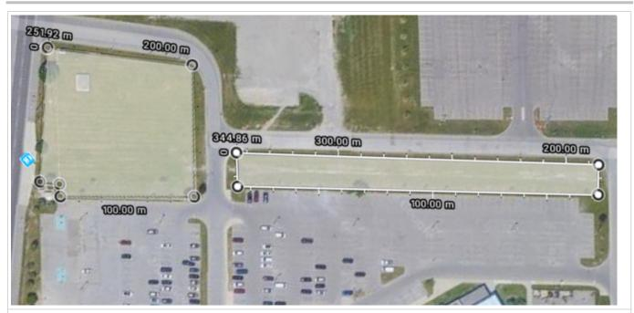
Figure D06.1- High Temp Loop Required Bore Hole Area
