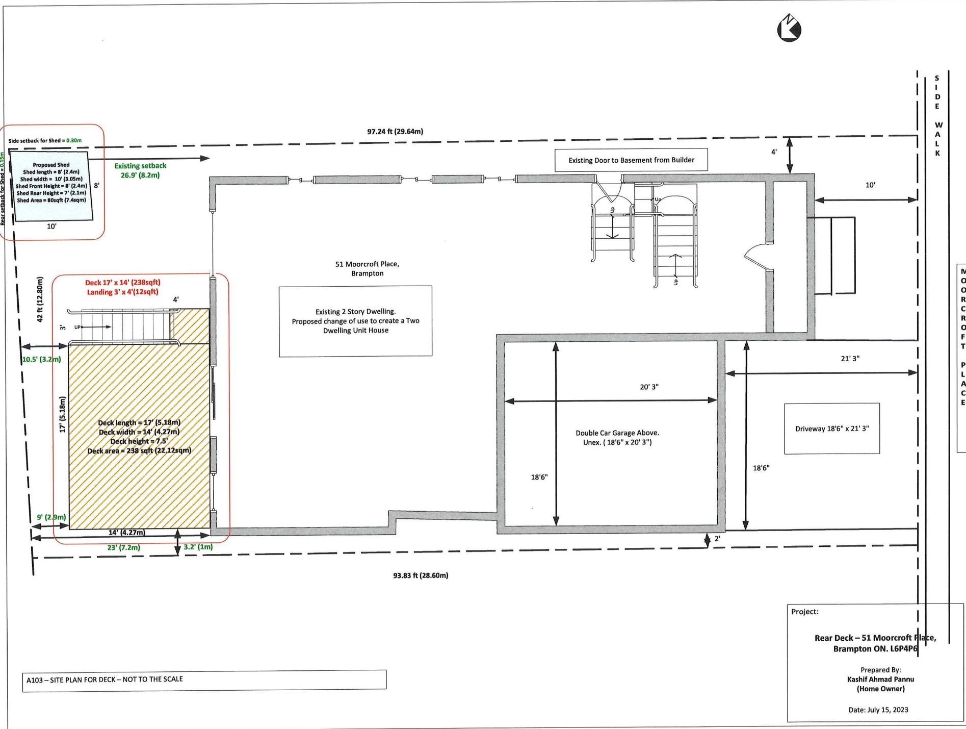
A103 – SITE PLAN FOR DECK – NOT TO THE SCALE
