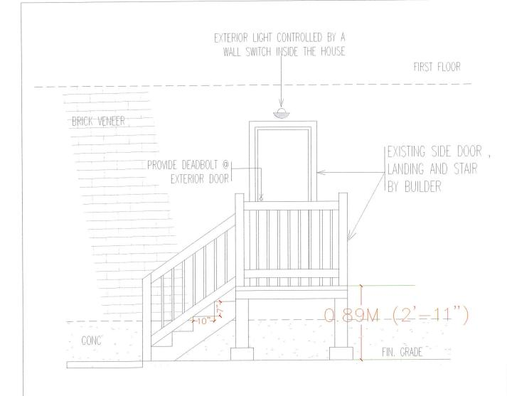
$\frac{\text{RHS ELEVATION WITH EXISTING SIDE DOOR, LANDING AND STAIR BY BUILDER}}{\text{SCALE}: \frac{1}{2} \quad \text{"} = 1 \text{'}}$
