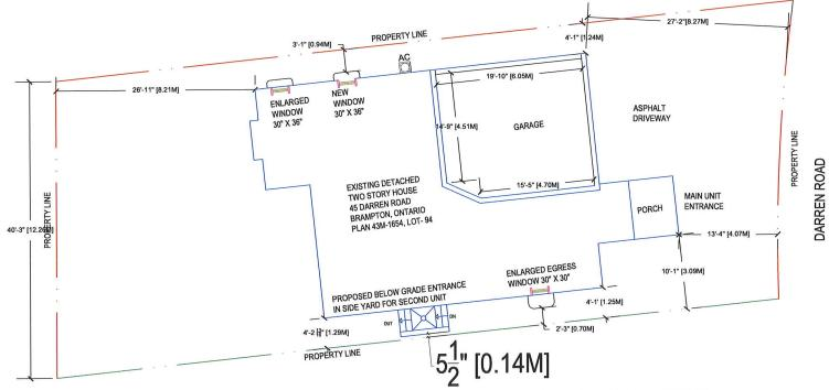
SCOPE OF WORK: PROPOSED BASEMENT APARTMENT (SECOND UNIT) 1 NEW WINDOW, 2 WINDOWS ENLARGEMENT AND PROPOSED BELOW GRADE ENTRANCE IN SIDE YARD FOR SECOND UNIT ENTRANCE
