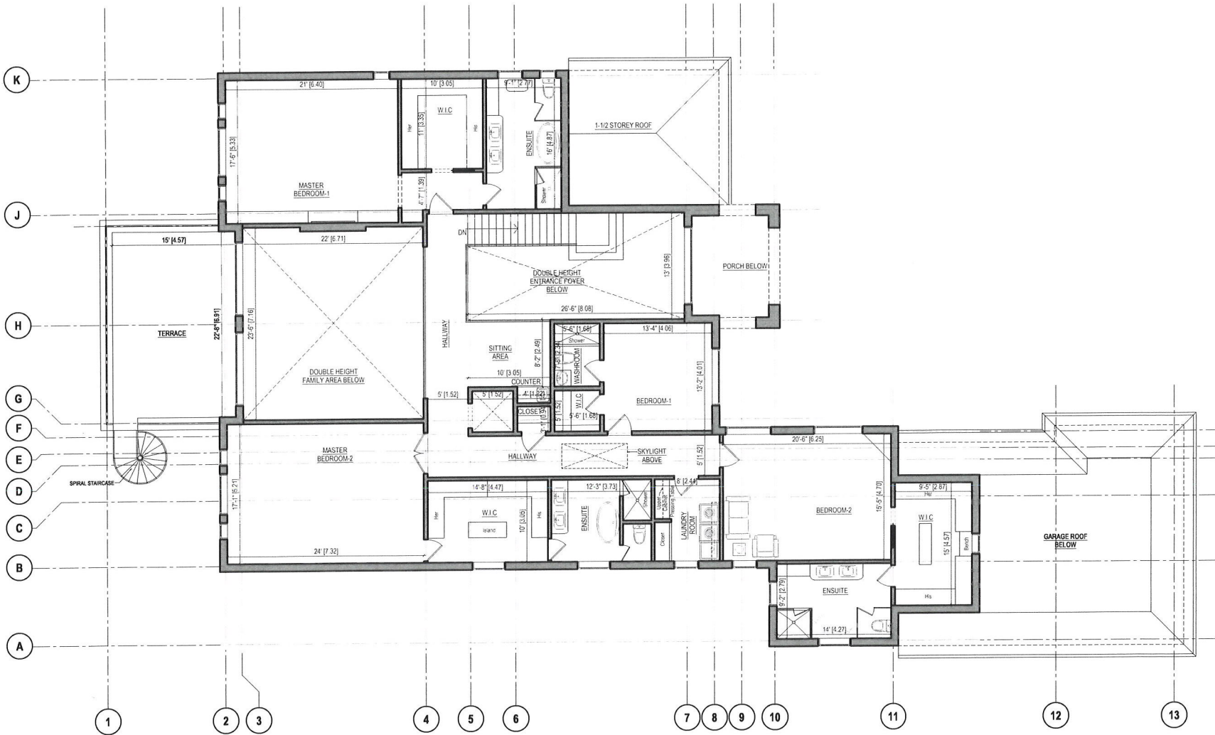
SECOND FLOOR PLAN Second Floor Area (including Double height): 4026.66 sq.ft. Double Height Area: 808.79 sq.ft.
