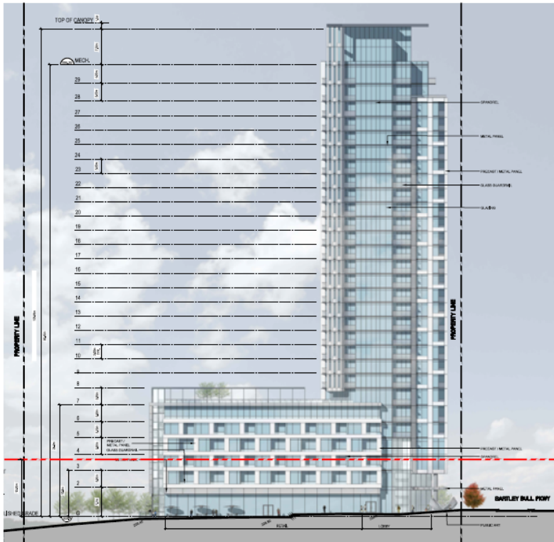
West Elevation (Main Street South Frontage)
