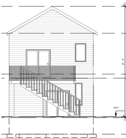
5.1.BB – Garage/Accessory Unit – Existing Rear (West) Elevation
