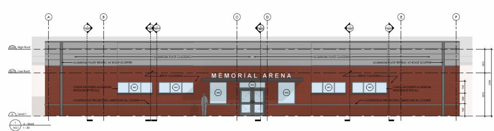
Figure 4: General composition of the west (main) elevation of the addition. The signage mounted on the canopy is proposed in the same font as the building signage on the north entrance pavilion (inset at right)
