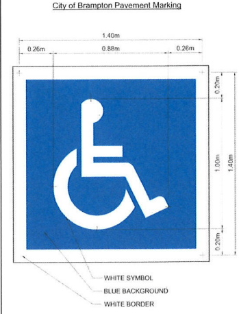
4 ACCESSIBLE PARKING SIGN SCALE: NTS
