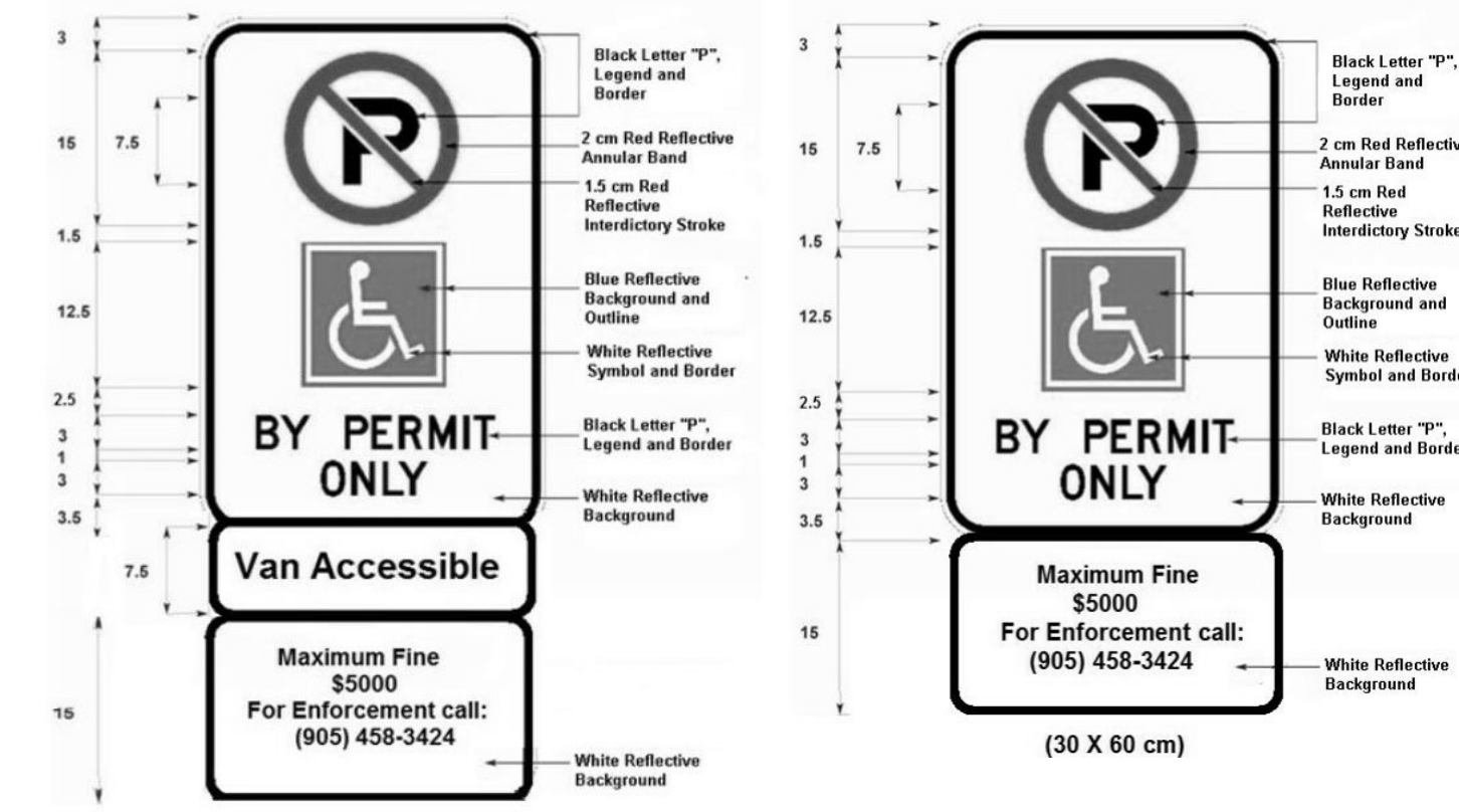
11.4 ACCESSIBLE PARKING SIGN DETAIL N.T.S.
