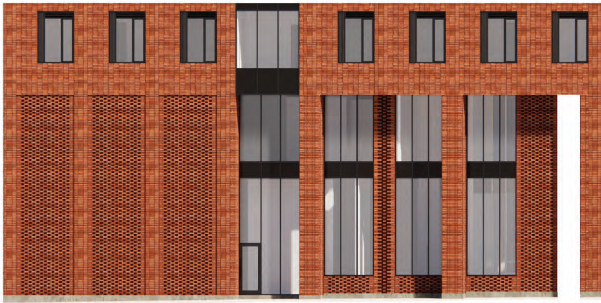
Proposed brick articulation strategy on the Mill Street North facade, which is designed in part to minimize the impact of a solid streetwall at the elevation's south end (Sweeny & Co Architects, 2024).
