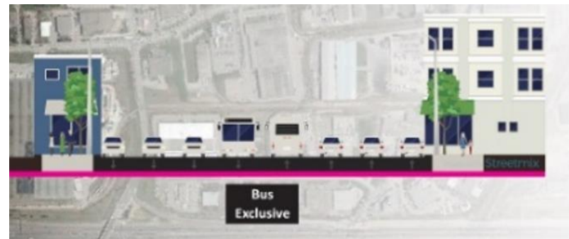
Sample road cross-section in-between Dixie Road and Highway 410 for Scenario 4 and Scenario 5
