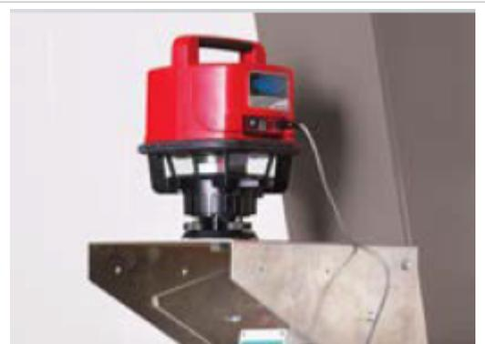
Figure E04.2 – Example of Laser Mount
