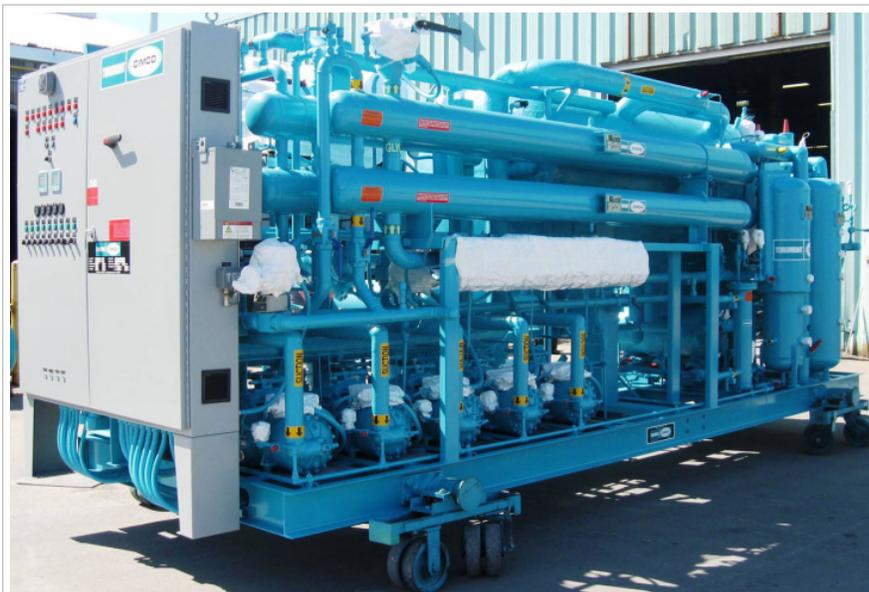
Figure E01.1 – Packaged Carbon Dioxide ice plant
