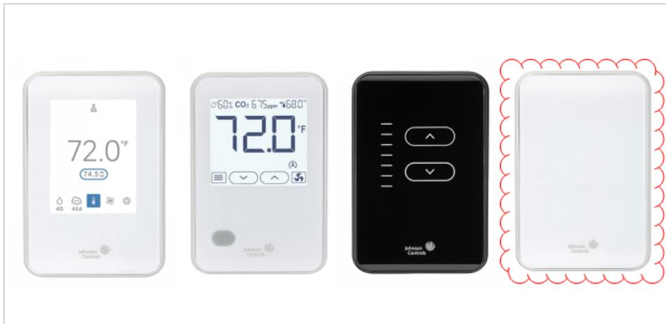
Figure C02.1 Depiction of the various networkable sensors (Johnson Controls power + BACnet MS/TP communications' SA-bus) available for connection to their VMA controllers.
