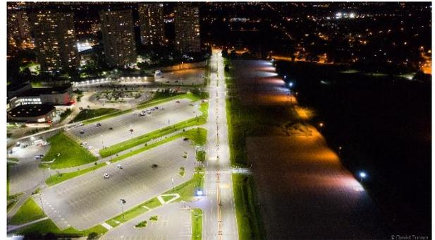
Figure A02.4 – A side by side comparison of LED (left) and metal halide/high pressure sodium (right, out of scope). This lighting retrofit was completed by MCW in 2019.
