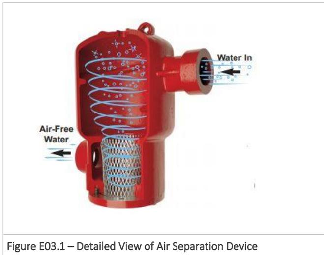
Figure E03.1 – Detailed View of Air Separation Device
