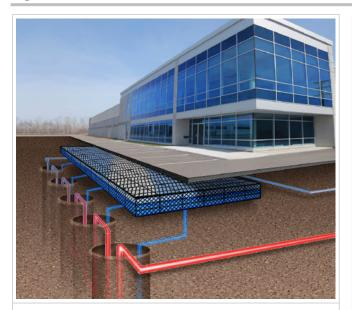
Figure D05.1- Ground Source Heat Loop
