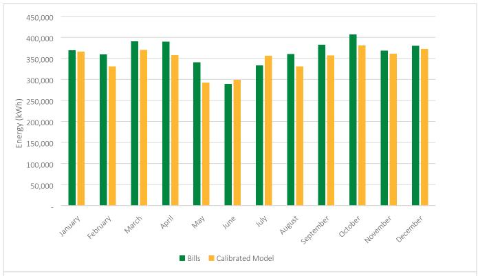
Figure 4.2.1: Electricity Calibration results for South Fletcher's Sportsplex
