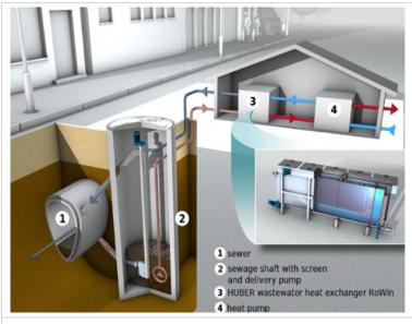
Figure D11.1- Principle of operation for a waste water source heat pump
