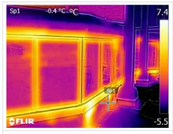
Figure G01.1— Thermal Imagine of existing windows indicating thermal bridging  $\,$
