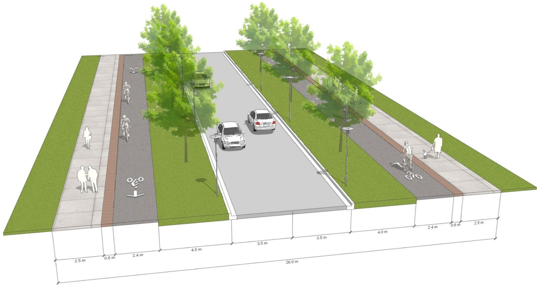
Figure 8. Street Section – 26.0m R.O.W., N.T.S.
