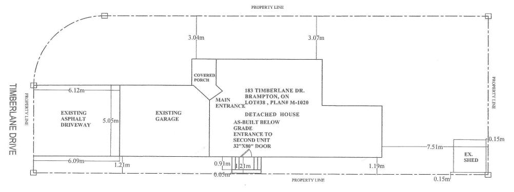
EXISTING MAIN FLOOR AREA: 55.33 m<sup>2</sup> EXISTING SECOND FLOOR AREA: 73.47 m<sup>2</sup> PROPOSED BASEMENT APARTMENT AREA: 47.72 m<sup>2</sup> PARKING SPACES REQUIRED: 2 SPACES
