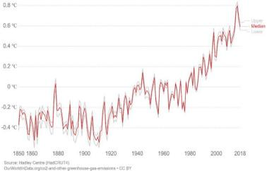
Measured in degrees Celsius (°C). The red lines represent the median average temperature change, and grey lines represent the upper and lower 95% confidence intervals.
