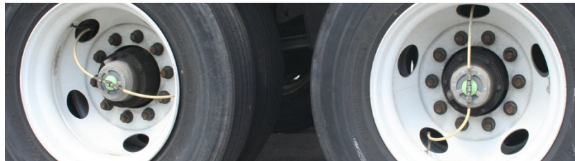
Figure 8: Automatic Tire Inflation System (courtesy NACFE)
