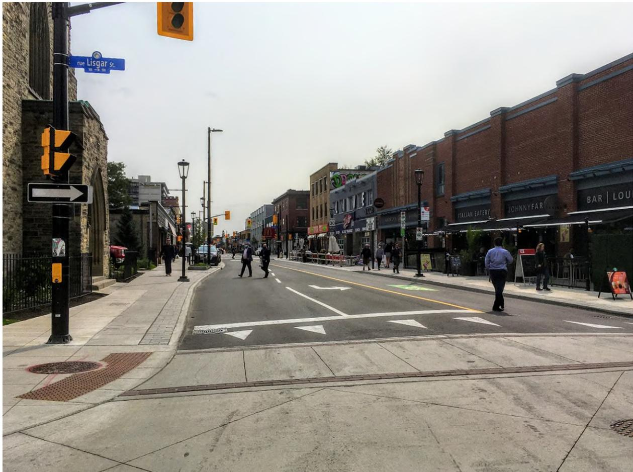
Figure 13: Ottawa's Elgin Street was recently reconstructed to a design speed of 30 km/h to improve safety for vulnerable road users (Credit: Matt Pinder)
