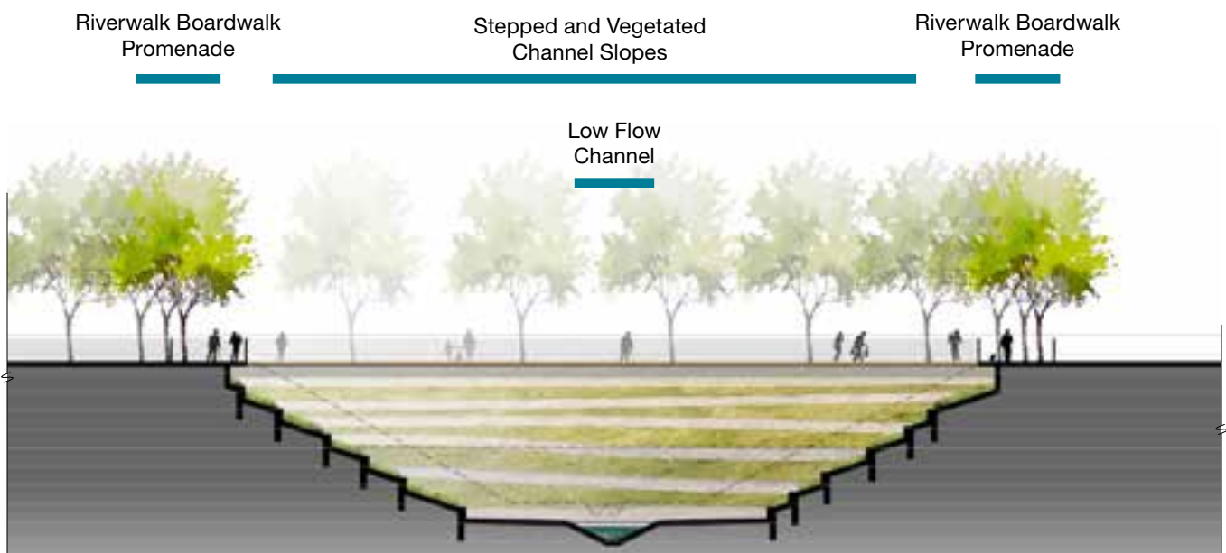
Fig. 246 Section Through Bypass Channel
