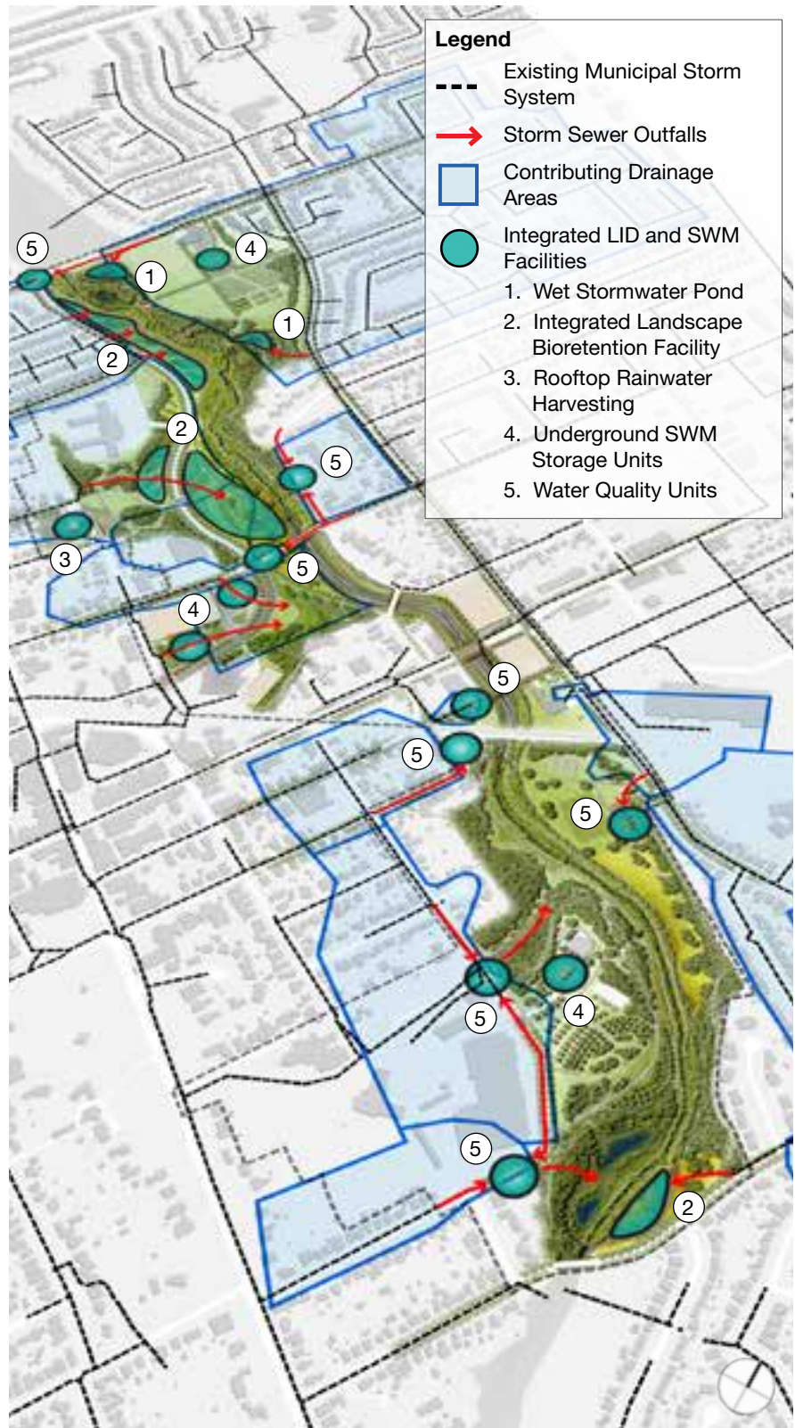
Fig. 104 Concept for Riverwalk Stormwater Management Strategy (to be assessed in future feasibility study)
