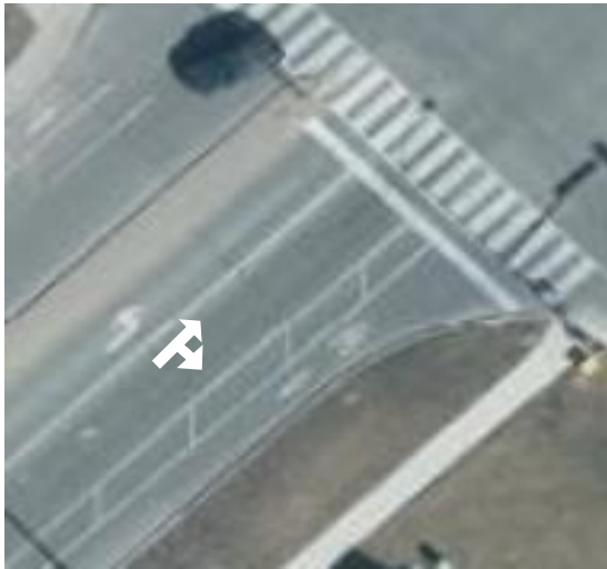
Directional arrows painted in lanes
