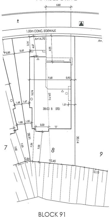
NOTE: BUILDER TO VERIFY LOCATION OF ALL HYDRANTS, STREET LIGHTS, TRANSFORMERS AND OTHER SERVICES. IF MIN, DIMENSIONS ARE NOT MAINTAINED BUILDER IS TO RELOCATE AT HIS OWN EXPENSE.
