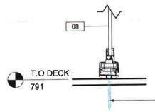
HECO TOPIX 8.0 x 100mm SCREWS INTO SOLID WOOD. 1 SCREW @ EACH PANEL JOINT
