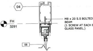
M8 x 20 S.S BOLTED INTO ALUMINUM (1 SCREW AT EACH END & 1 SCREW PER GLASS PANEL.)
