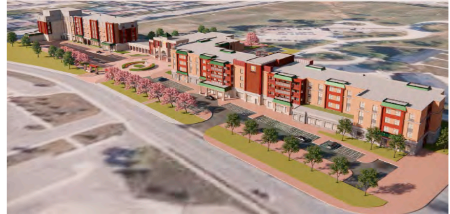
View of Academic Drive frontage, showing front-yard setback lined with trees, circular parking and 3-section linear mass extending to the south of the property from Queen Street West. (IBI Architects)
