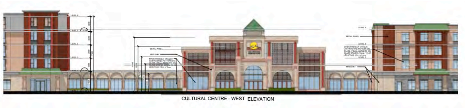
West elevation showing central amenity building connected with one-storey link to the north (5-storey) and south (4-storey) residential components.
