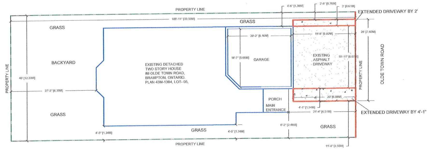
SCOPE OF WORK: DRIVEWAY WIDTH EXTENSION FROM 19'-11" TO 26'-00"
