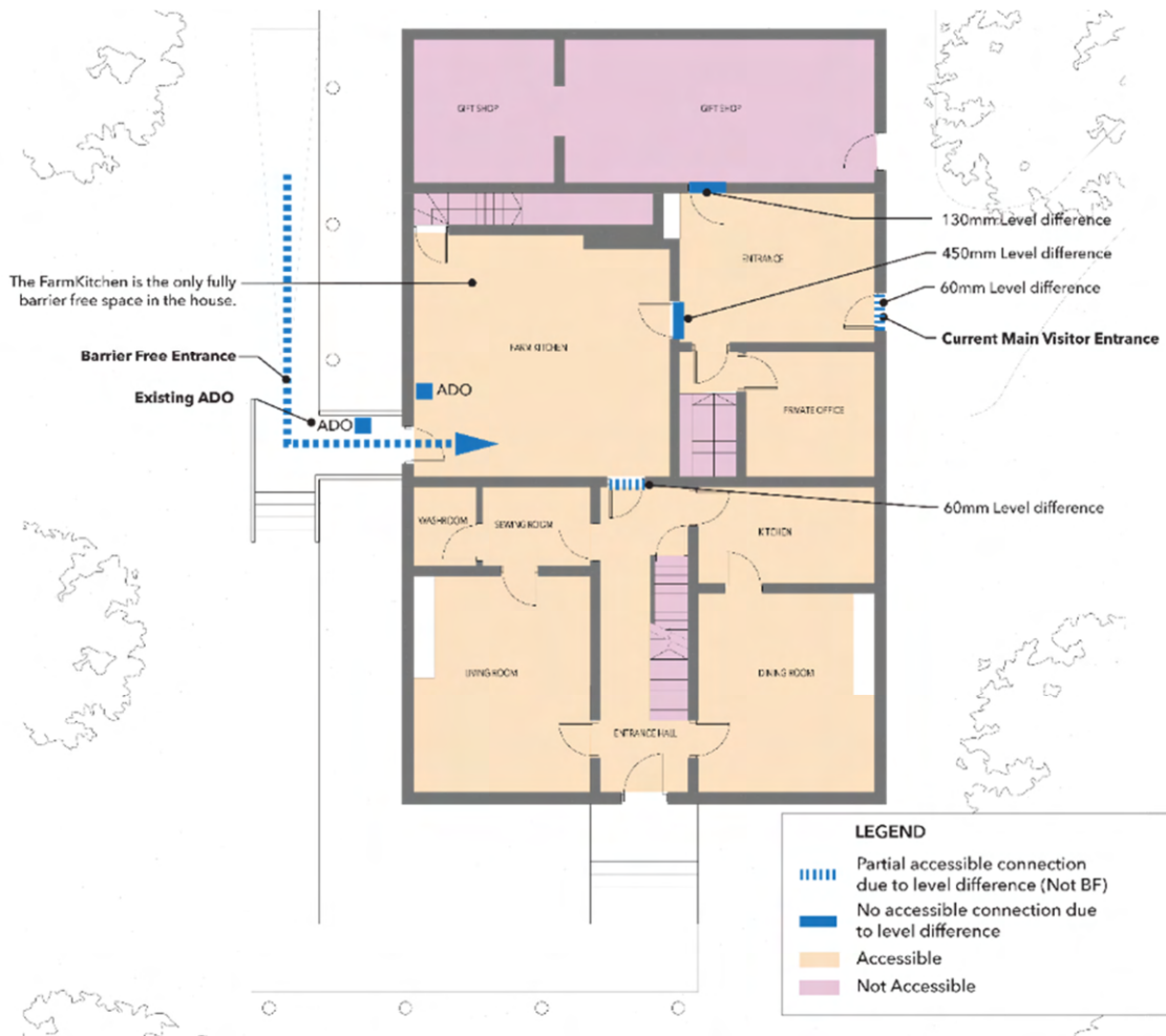
Figure 24: Existing accessibility in the Main House Above: Ground Floor Left: Second Floor
