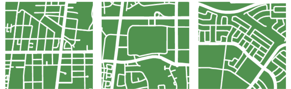
Figure 3.27. Block Pattern and Network Connectivity. Six examples from different parts of Brampton. Note the higher amount of possible routes in some parts of the city than others. The greater the number of intersections in a given area, the more connected and complete the network.
