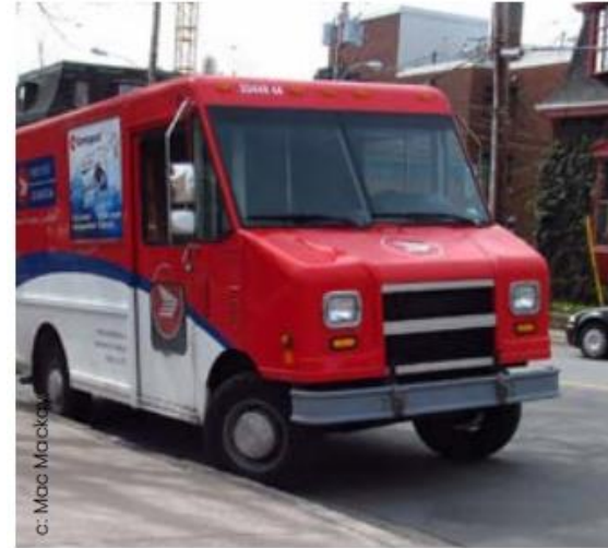
Figure 3.9. Design vehicles are the most common large vehicles that use city streets, similar to a Canada Post or other courier trucks.
