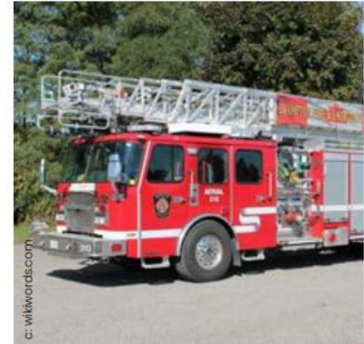
Figure 3.10. Control vehicles, like fire trucks, are the largest vehicles that use city streets. They are permitted to use more of the street to maneuver.
